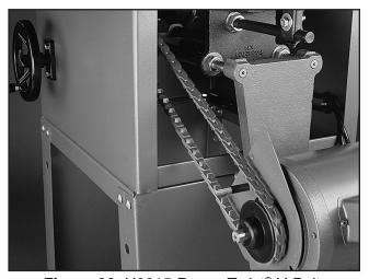
Figure 36. H9815 Power Twist® V-Belt.
